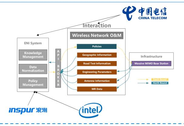
✓ PoC Project Goal: Data Analysis and Policy-Based Coverage Optimization. Demonstrate the use of AI based data analysis to enable policy-based coverage optimization for Massive MIMO BS.
