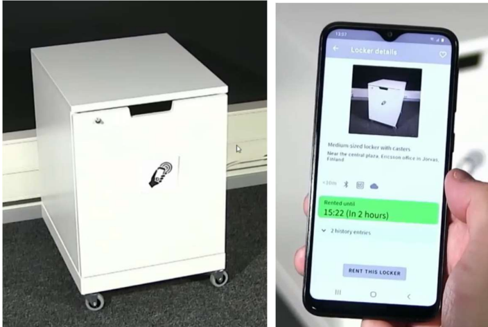
Figure 1: Physical demonstration locker with Raspberry Pi single board computer controller (left), and the Android mobile phone application used to rent and access lockers.
