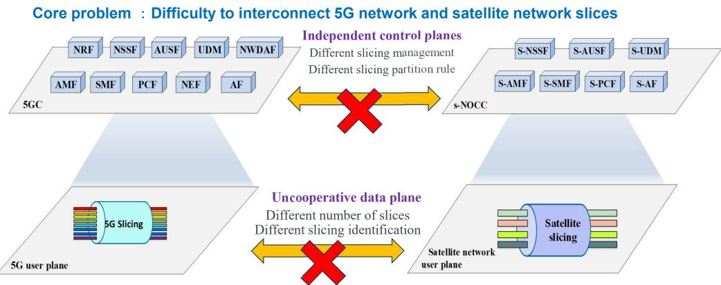
Core problem : Ground mobile communication network and space satellite network are different on service classification of network slicing, number of slices and slicing construction. As a result, the slices of the two networks cannot be directly interconnected.
