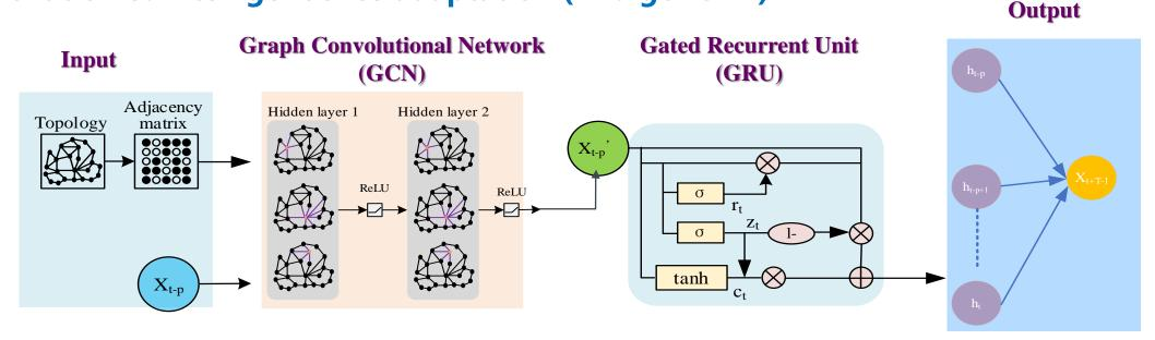
To construct differentiated network slices involving different service characteristics, and realize multi-service integration, an intelligent slice mapping mechanism based on spatial-temporal correlation is proposed based on Graph Convolutional Network (GCN) and Gated Recurrent Unit (GRU).
