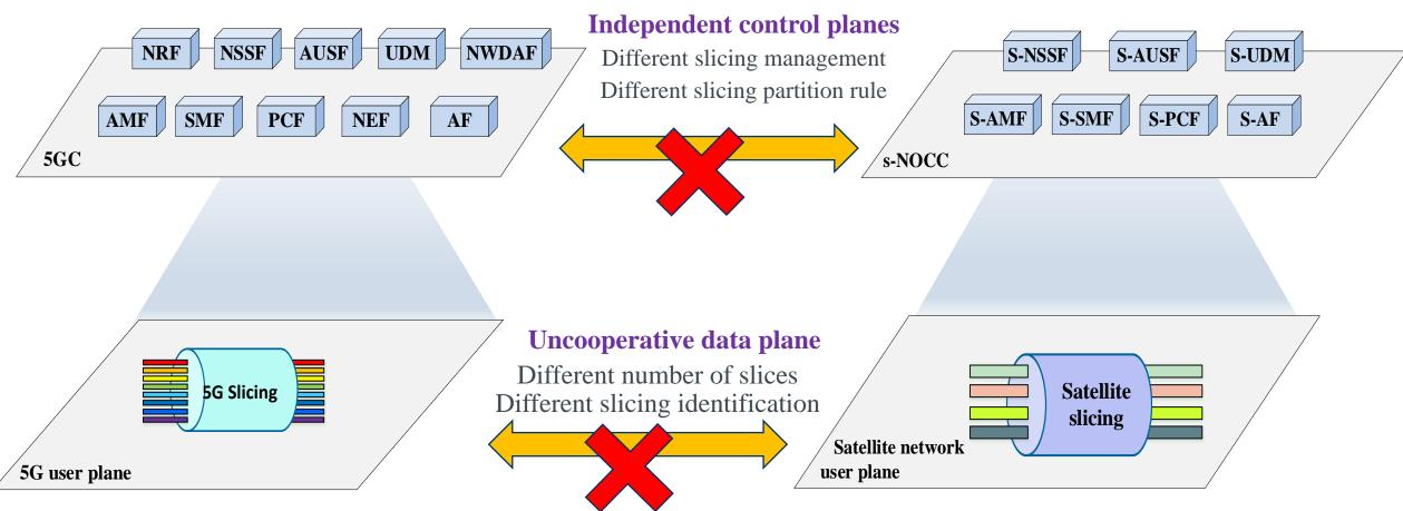
**Core problem**: Ground mobile communication network and space satellite network are different on service classification of network slicing, number of slices and slicing construction. As a result, the slices of the two networks cannot be directly interconnected.
